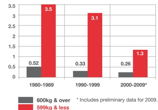
Fig. 3 Stall/spin accident rates per 100,000 flying hours for the two weight categories
