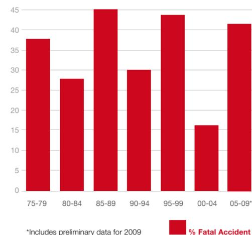
Fig. 2 Aeroplanes of 5,700 kg & less, stall/spin accidents as a percentage of all fatal accidents
