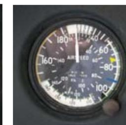
Fig. 8b Aeroplane ASI with 'CS22 markings' added
